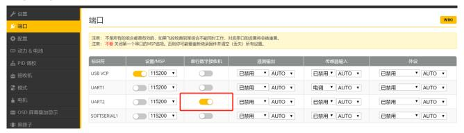
Set up protocol for receiver (SBUS protocol choose SBUS, FPORT protocol choose FPort, either-or)
